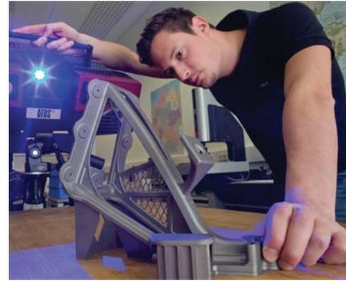
Taking optical measurements of a lightweight structure (source AKTIV Karmann).
